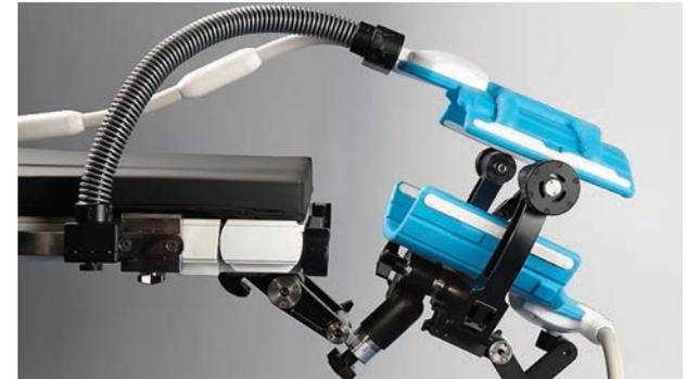
Integrated head fixation and flexible imaging coils maximize surgical access and iMRI image quality.
